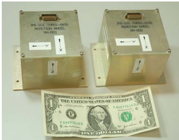
IMI-101 Flight Units to be flown on AFRL's University Nanosat 4 CuSat in 2009
